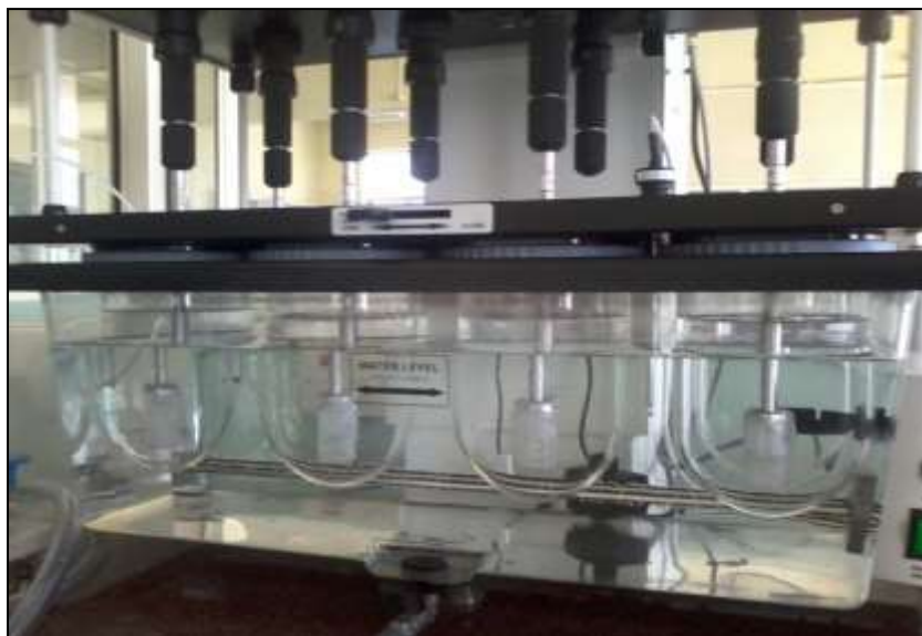
Figure 2: Dissolution test apparatus of in-vitro drug release
